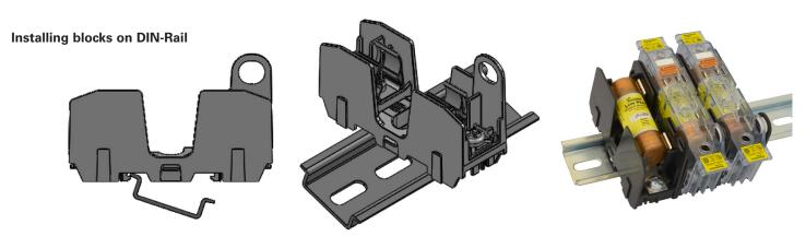
Place one edge of DIN-Rail in fuse block base, then rotate block down until it clicks into place.
