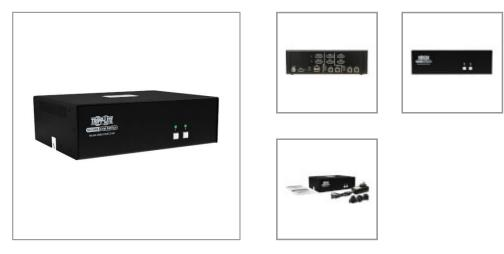
NIAP-certified KVM lets you access multiple computers from a single console while protecting data from accidental or unauthorized transfer between them.
