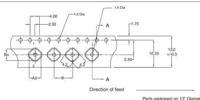
Parts packaged on 13" Diameter reel, 4,150 parts per reel.
