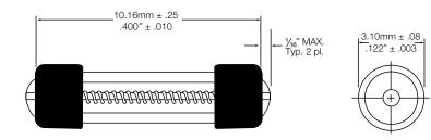
CATALOG SYMBOL: TEL-350mA VOLTAGE RATING: 600V DC INTERRUPTING RATING: 6A DC, Battery Source INTERRUPTION TIMES: 4 hrs. min. @ 100% of rated current (350mA) 210 sec. max. @ 150% of rated current (525mA) PHYSICAL SIZE: 3mm x 10mm CONSTRUCTION: Glass tube Nickel-plated brass end caps AGENCY INFORMATION: UL Recognized, Guide No. JDYX2, File No. E19180
