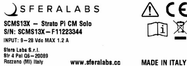
EXAMPLE RATING AND IDENTIFICATION PLATE
