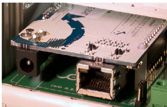
AN ARDUINO BOARD WITH PINS AND TURRETS PROPERLY ALIGNED
