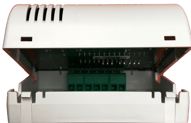
ALIGN THE CONNECTION PINS WITH THE TERMINAL BLOCK
