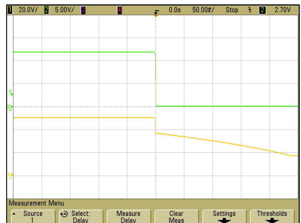
Figure 4: ADQ800-48S12B Output voltage shut down by power Off (2mS/div)
