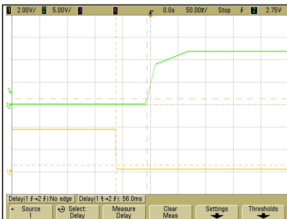
Figure 5: ADQ800-48S12B Output voltage startup by remote ON (20mS/div)
