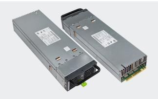
Advanced Energy's Artesyn HPS3000 series bulk front end AC-DC power supply accepts a wide range 90 to 264 VAC input and provides a main 48 V output plus a 5 V standby output. It has a full load efficiency of more than 90% and is rated at 3,000 watts when operating from a nominal 200 VAC input. Housed in a 1U x 4.2 inch form factor enclosure, the power supply has a power density of 40 watts per cubic in; four units can fit on a standard 19 in rack shelf, to provide a total of 12 kilowatts.
