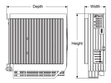
Design may change when using a fan and/or rated current > 350 A
