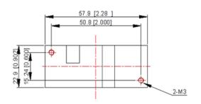
$\begin{tabular}{lll} UNIT: mm[inch] & BOTTOM VIEW: pin on upside \\ TOLERANCE: X.Xmm $\pm 0.5 mm[X \times in. \pm 0.02in.] \\ & \times XXmm $\pm 0.25 mm[X \times X in. \pm 0.01in.] \end{tabular}$
