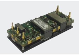
Advanced Energy's Artesyn AVO240 series eighth-brick isolated DC-DC converter is designed specifically to provide a regulated low noise 12 Vdc output for feeding downstream non-isolated point-of-load (POL) converters in systems with distributed power architectures (DPA). Rated at 240 watts, it can deliver up to 20 amps. The converter has a wide input range of 41 to 75 Vdc and is designed primarily for use with standard 48 V telecommunications equipment supplies.
