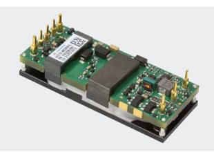
Advanced Energy's Artesyn AVO100 series of eighth-brick isolated DC-DC converters comprises six single output models offering fully regulated voltages of 1.2 V, 1.5 V, 1.8 V, 2.5 V, 3.3 V or 5.0 V. These converters can deliver up to 50 amps and up to 100 watts of output power, depending on the particular model. They have a wide 2:1 input range of 36 to 75 Vdc and are designed primarily for use with standard 48 V telecommunications equipment supplies.
