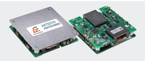
Advanced Energy's Artesyn ADH700 series half-brick isolated DC-DC converter provides a single regulated low noise output. ADH700-48S28 with 28V/25A output and ADH700-48S50 with 50V/14A output. It has a Telecom input range of 36 to 75Vdc and is designed primarily for use with standard 48 V telecommunications equipment supplies. The converter's main application area is in low power and remote radio head (RRH) telecommunications applications.
