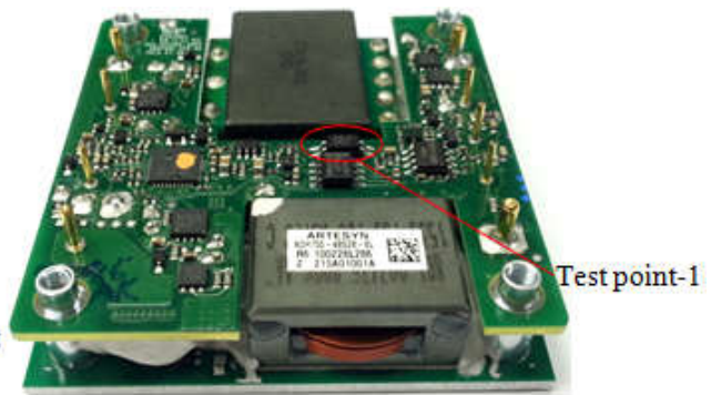
Figure 12: Temperature test point-1
