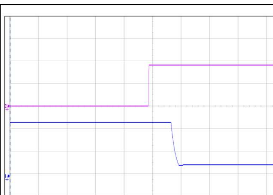
Figure 6: AVO120-48S12 Output Shutdown by Remote Off (100ms/div)
