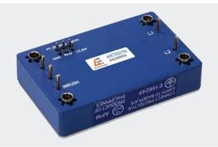
The AIQ00ZPFC series quarter-brick power factor correction module accepts a 100–122 Vac input and presents a unity power factor. It accommodates AC supply frequencies in the range 360 to 800 Hz. Rated at 75 watts, the module offers a power conversion efficiency of up to 90% and provides a typical output voltage of 393 Vdc.
