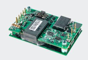
Advanced Energy's Artesyn AGQ500 series Quarter-brick isolated DC-DC converters provides a single, regulated and low noise output. The AGQ500-48S50 has a 50V/10A output. It has a Telecom input range of 36 to 75 Vdc and is designed primarily for use with standard 48 V telecommunications equipment supplies. The converter's main application area is in low power and remote radio head (RRH) telecommunications applications.
