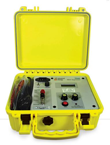
The Model R1M-A series portable megohmmeter is designed to measure very high values of insulation resistance The instrument has six resistance ranges from 1 M $\Omega$  full scale to 100 G $\Omega$  full scale, with 100 % overrange capability. Four test voltages of 50, 100, 250, and 500 VDC are provided (50 V maximum to be used with resistances less than 1 M $\Omega$ ). Resistance readings are displayed on a 3½ digit LCD display with 0.5 inch character height.
