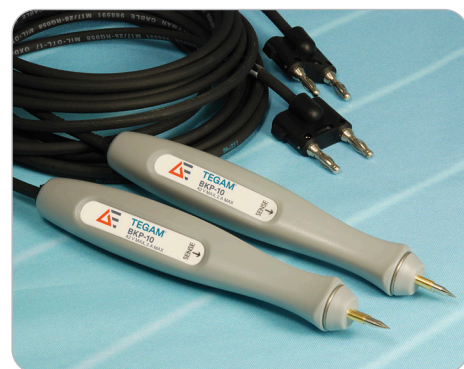
TEGAM BKP-10 Kelvin probes used to measure contact resistance between shunt and circuit board trace
