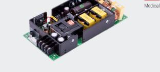
Advanced Energy's SL Power MINT2270 medically-approved AC-DC power supplies have dual output - 5 V and 24 V, delivering up to 270 Watts convection output power. It has universal 90 to 264 Vac input voltage range and up to 90% typical efficiency, which support AC OK, DC OK as well as Remote On/Off signals.
