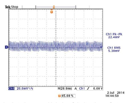
To verify that the output ripple and noise does not exceed the level specified in the product specification, measured using a scope probe socket with 0.1uF ceramic and a 10uF electrolytic capacitor connected in parallel across it, 20MHz BW.
