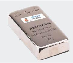
Standard features include 1,500 Vdc input/output isolation and short-circuit protection with auto-restart. AEE series converters have an operating temperature range of -40 to 71°C without derating and are suitable for diverse applications in areas such as industrial automation, instrumentation, test and measurement, and telecommunications. The 3.3 Vdc output model has a power output rating of 13.2 watts, while all other models are rated at 15 watts.
