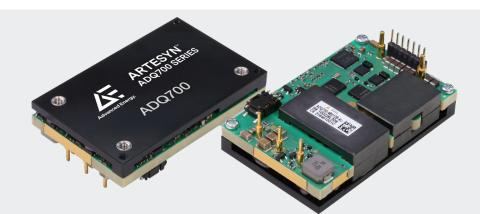
ADQ700 series quarter-brick isolated DC-DC converters produce a single fully regulated 12 V output and rated at 700 W, these converters can deliver up to 58 A output current and have no minimum load requirement. They have an input voltage range of 40 to 60 V and are primarily designed for use with standard 48 V supplies in computing and server applications, as well as regulated 48V supplies in communications equipment.
