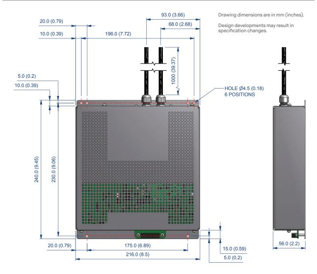
MOUNTING: 6 OFF M4 CLEARANCE HOLES IN BASE AS SHOWN.
