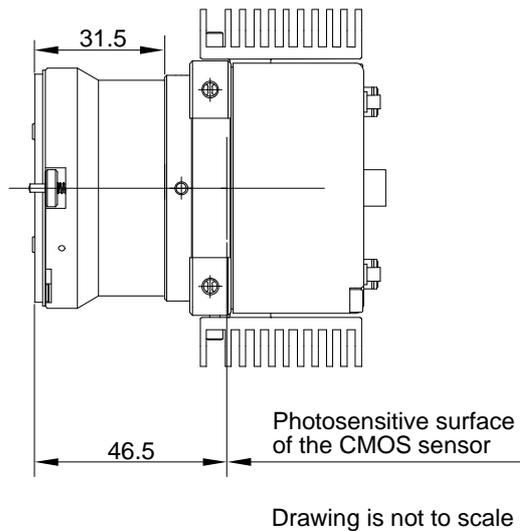
Fig. 5: Camera with F-mount Adapter Attached (in mm; 2k and 4k Cameras)
