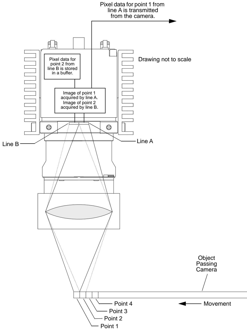
Fig. 13: Dual Line Acquisition - ExSync Cycle 1
