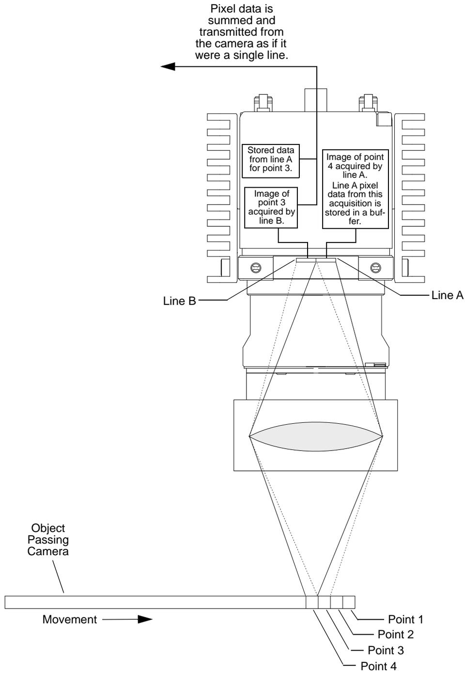
Fig. 21: Time Delayed Line Summing - Acquisition Four
