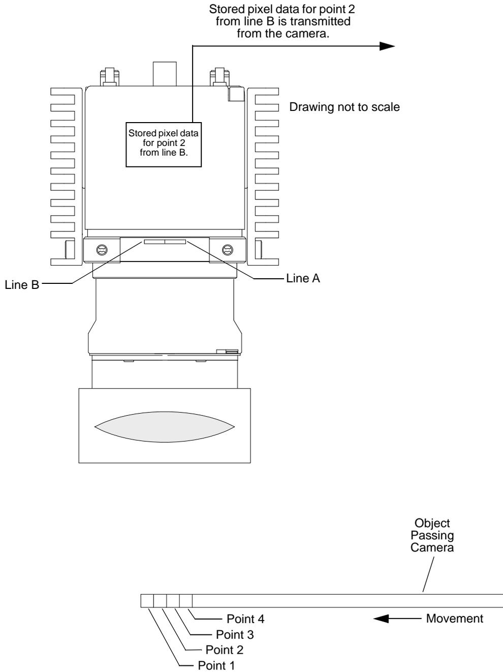
Fig. 14: Dual Line Acquisition - ExSync Cycle 2
