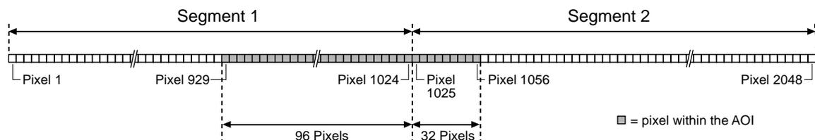
Fig. 31: AOI Falling Across Segments - Horizontal Binning Enabled
