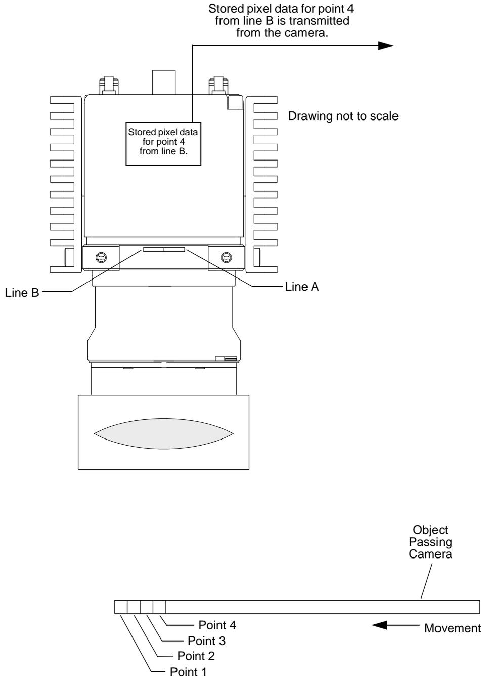
Fig. 16: Dual Line Acquisition - ExSync Cycle 4
