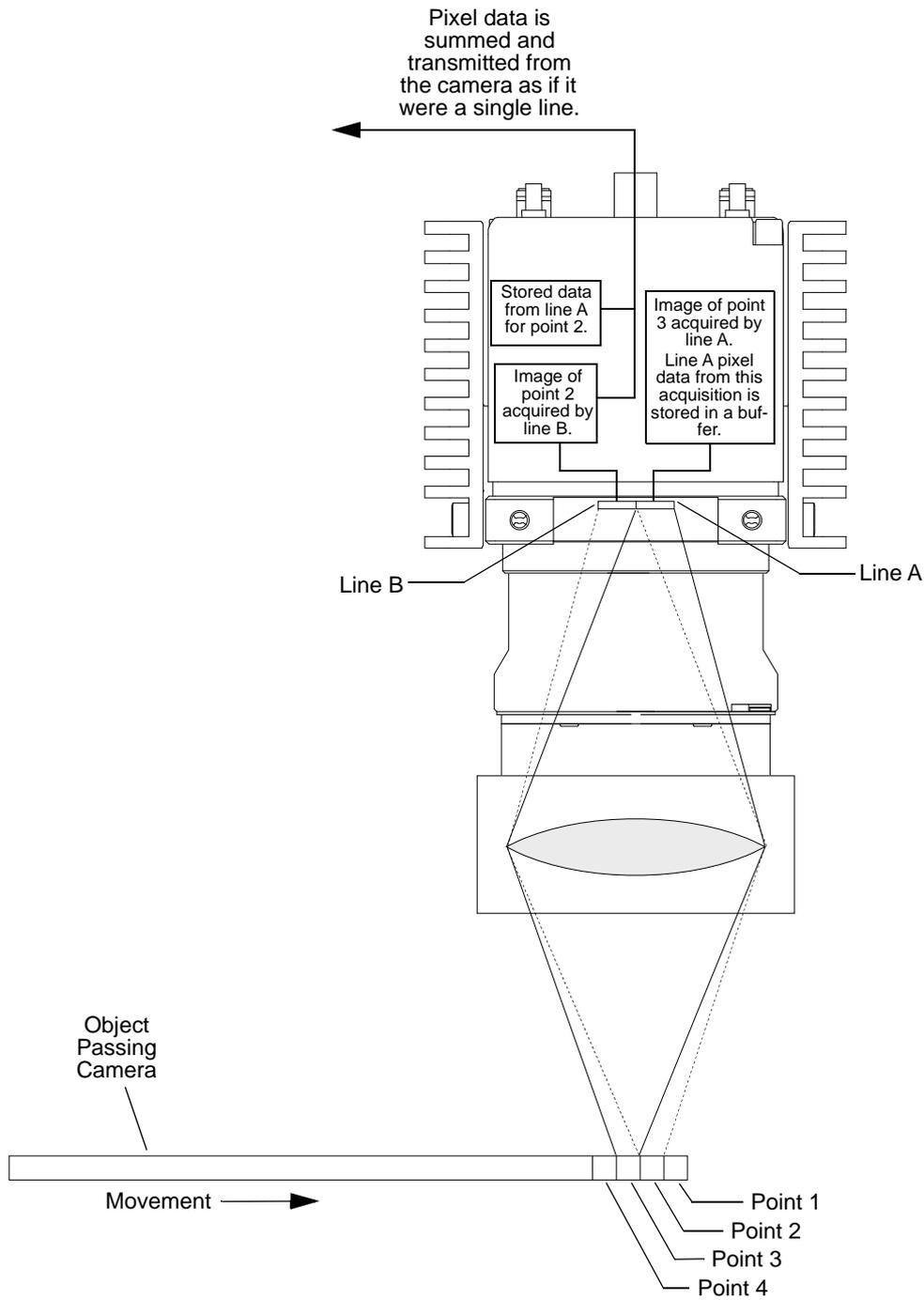
Fig. 20: Time Delayed Line Summing - Acquisition Three
