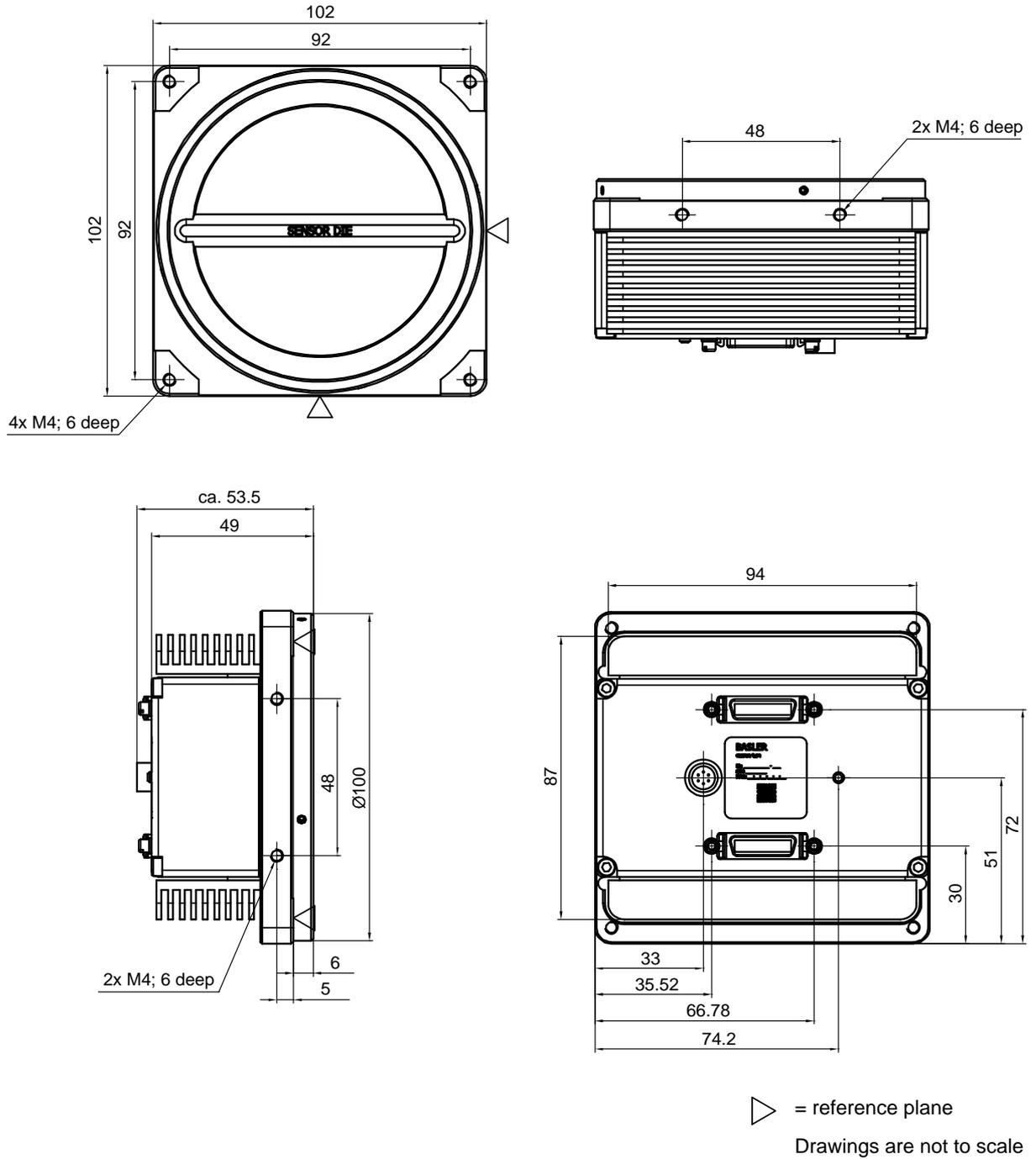
Fig. 6: Mechanical Dimensions (in mm; 8k Cameras)
