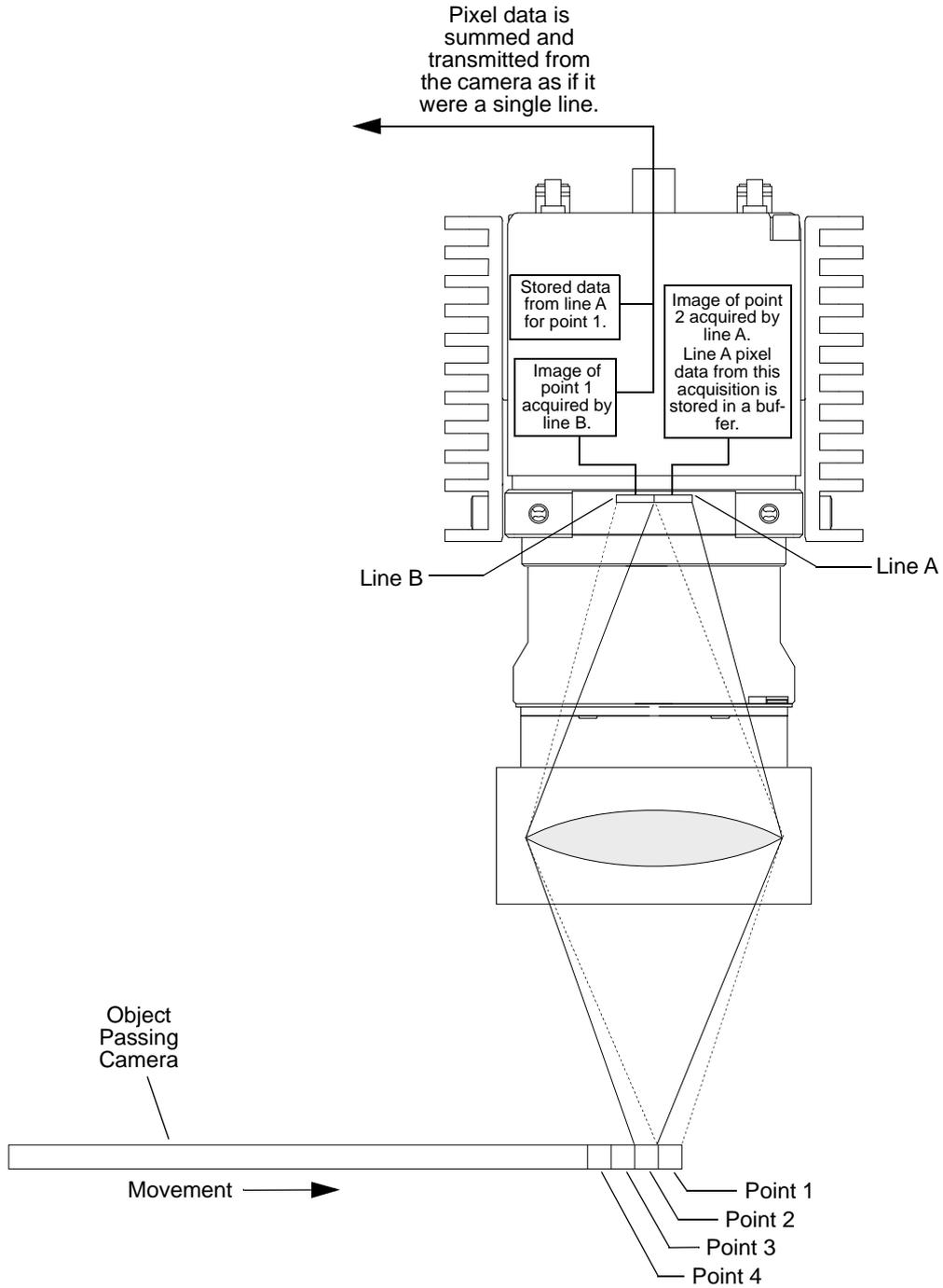
Fig. 19: Time Delayed Line Summing - Acquisition Two
