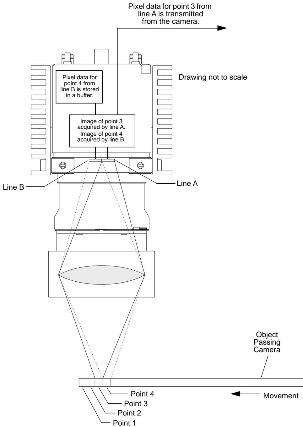
Fig. 15: Dual Line Acquisition - ExSync Cycle 3
