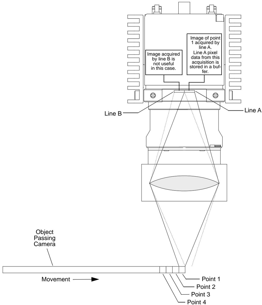
Fig. 18: Time Delayed Line Summing - Acquisition One
