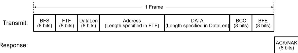
Fig. 50: Representation of a Command Frame and Response
