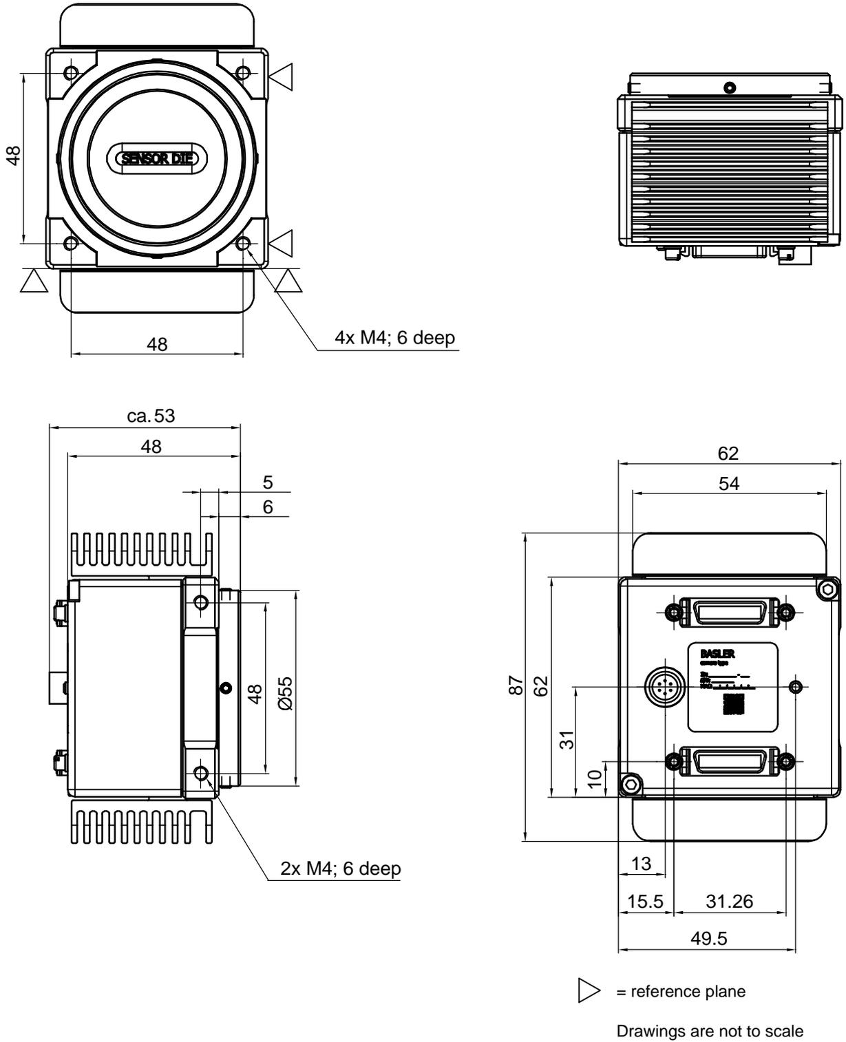
Fig. 2: Mechanical Dimensions (in mm; 2k and 4k Cameras)
