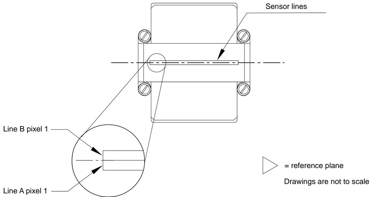
Fig. 4: Sensor Line Location (2k and 4k Cameras)
