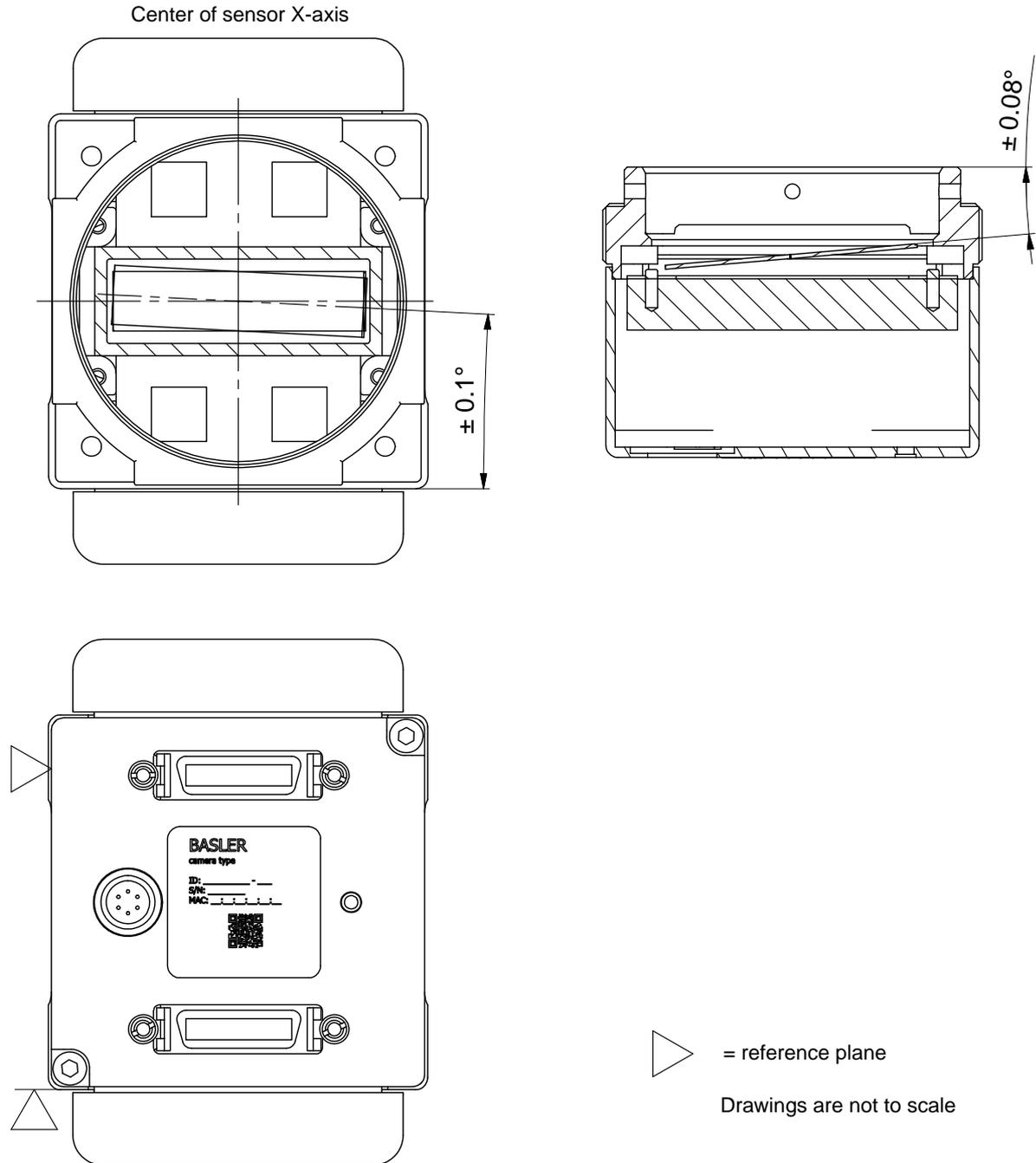
Fig. 3: Sensor Positioning Accuracy (in mm unless otherwise noted; 2k and 4k Cameras)
