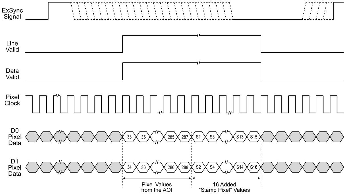
Fig. 48: Stamp Pixels with 2 Tap Video Data Output, Edge or Level Controlled Exposure, and an AOI
