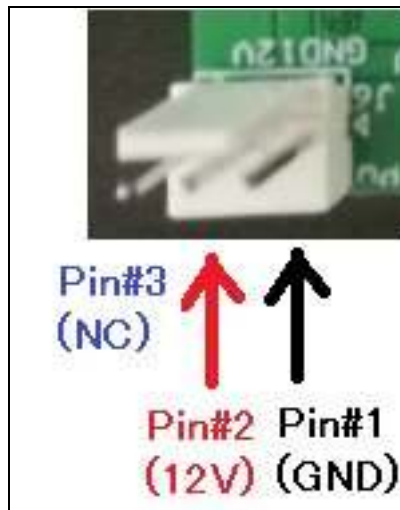
Figure-5: J6 pin header for 12V cooling fan
