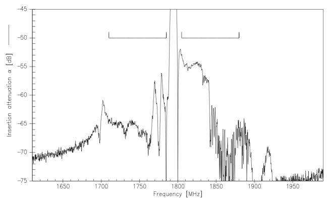
Frequency Response Tx-Rx (differential mode, wideband)
