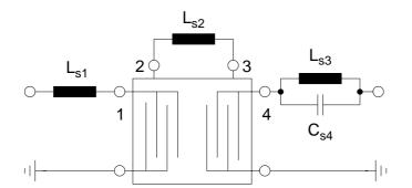
$L_{s1} = 24.0 \text{ nH}$   $L_{s2} = 36.0 \text{ nH}$   $L_{s3} = 19.0 \text{ nH}$  $C_{s4} = 0.50 \text{ pF}$
