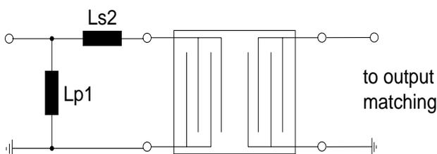
**Fig. 3 shunt L – series L matching**
