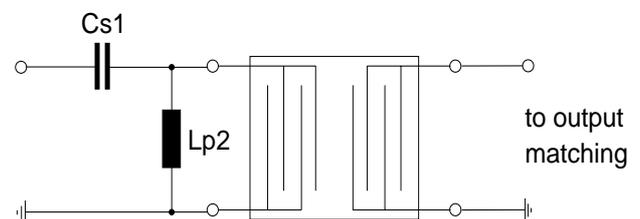
**Fig. 4 series C – shunt L matching**
