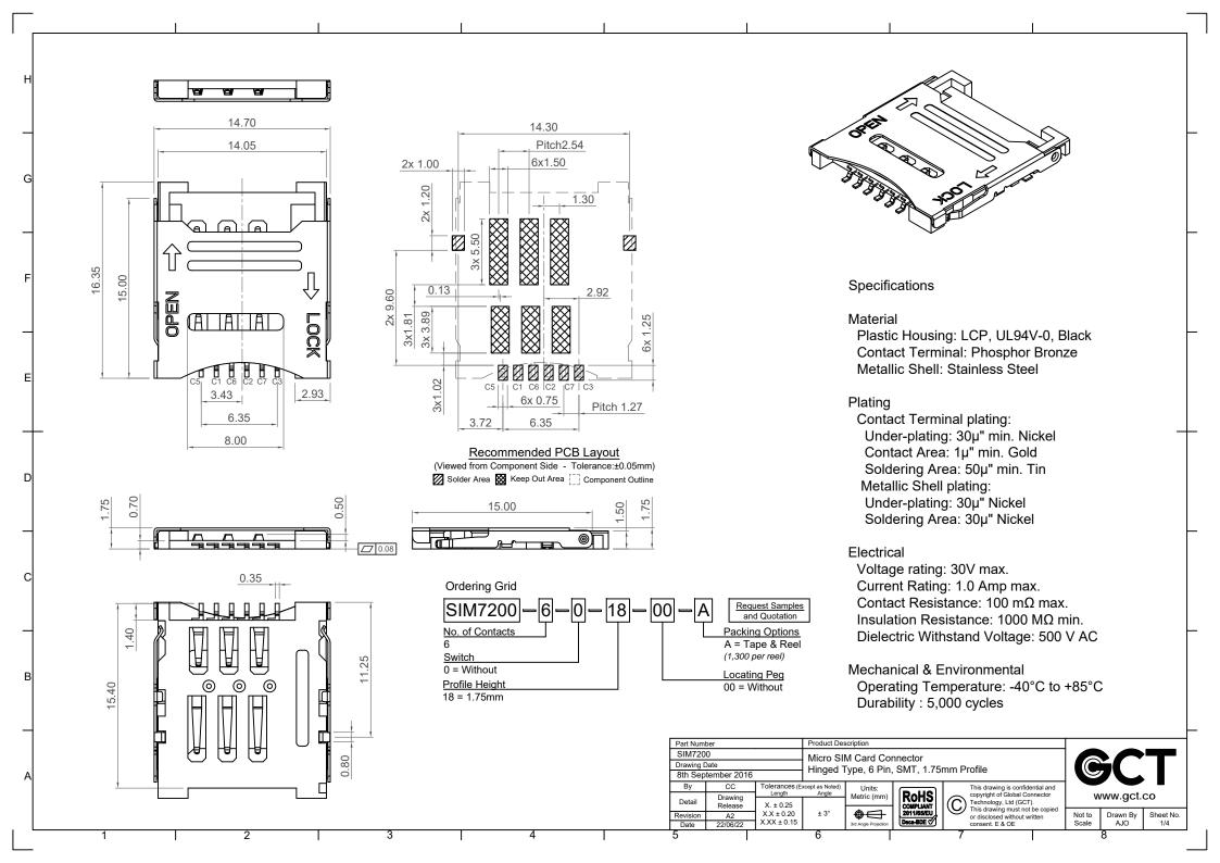
Slide metal lid from 'LOCK' position Open metal lid to allow Micro SIM card to be inserted to 'OPEN' position Place Micro SIM card against contacts, chip face down Close metal lid and slide back to 'LOCK' position Part Number Product Description SIM7200 Micro SIM Card Connector Drawing Date Hinged Type, 6 Pin, SMT, 1.75mm Profile 8th September 2016 This drawing is confidential and copyright of Global Connector RoHS COMPLIANT 2011/65/EU Drawing Technology, Ltd (GCT).
