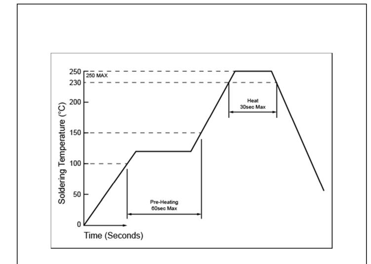
Fig. 1. Recommended Reflow Temp. Profile
