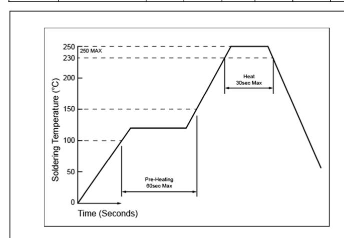
Fig. 1. Recommended Reflow Temp. Profile
