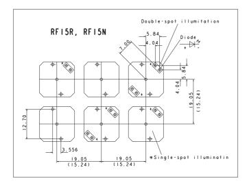
View on component side All hole diameters 1.1 +/- 0.1 mm PCB layout keyswitch 1/400" grid
