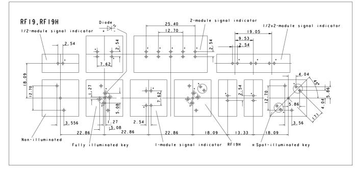
\*The LED may be positioned either on the left-hand or right-hand side. Standard version: LED on left-hand side View on component side, all hole diameters 1.1 +/- 0.1 mm
