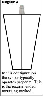
As the bin increases in size, the less likely the installation is going to detect unwanted objects and noise.
