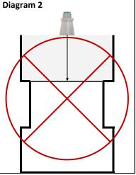
In both of these configurations the sensor will range to the first indentation in the trash bin. The indentation creates a large detectable reflection.
