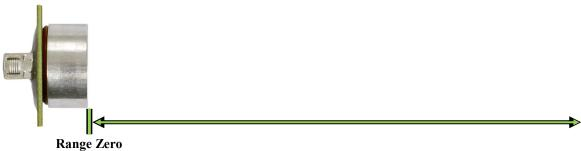
The range is measured from the front of the transducer to the target.
