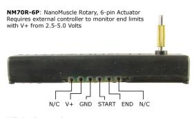
N/C: Not Connected START: HIGH (V+) when actuator is at rest END: HIGH (V+) when actuator is at end of stroke Note: No safe capability: do not over heat SMA wires
