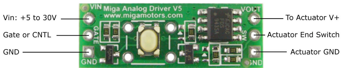
Miga Analog Driver V5 -Pinout Diagram
