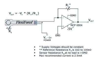
In the circuit shown, the dynamic force range of the sensor can be adjusted by changing the reference resistor  $(R_F)$  or by changing the Drive Voltage  $(V_0)$ . Refer to the <u>Saturation</u> section for additional information.
