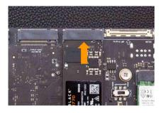
• Install a compatible wireless network module to the M.2 E key socket. Then assemble the WiFi/BT Antennas. Please refer to Mutiple Internet Connections section for a list of compatible modules. If you don't need a wireless connection, you can skip this step.
