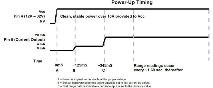
**A.** Power-Up timing begins when a voltage above 10V is maintained for the sensor.
