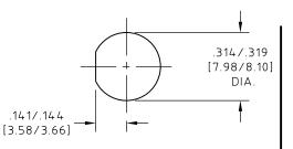
PANEL CUT OUT HUBER+SUHNER Astrolab REFERENCE "PC4" TORQUE MOUNTING NUT TO 20±2 IN-LBS [2.96±.3 Nm]
