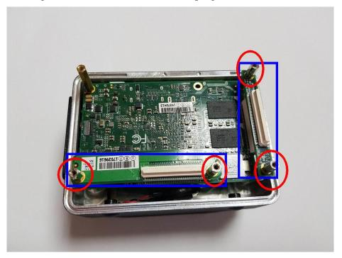
4. Put the NET plus board to be directed into the spacers and the standoff well.
