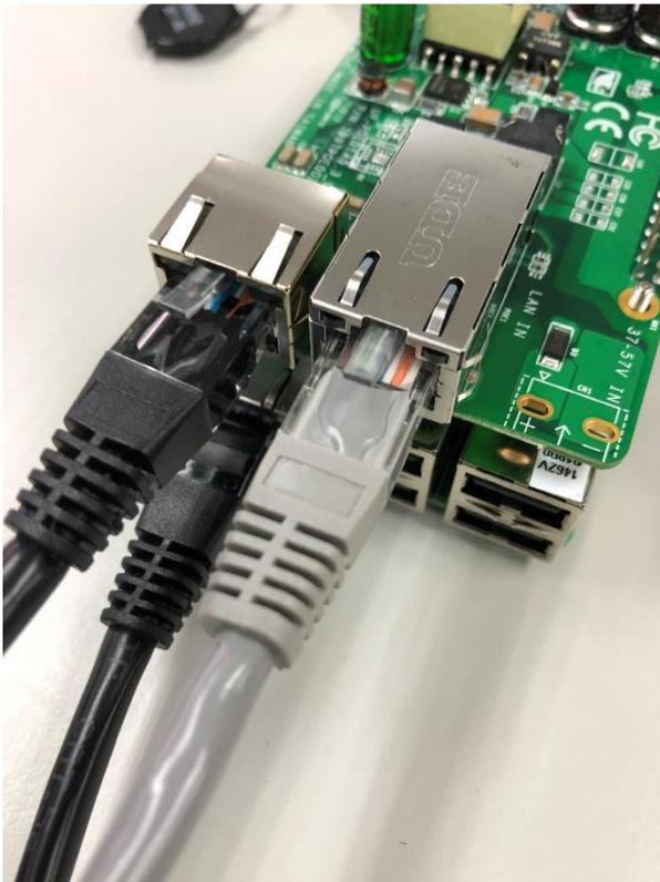
7. PoE board will power your MB through 40PIN header and transmit LAN signal to your MB via LAN cable
