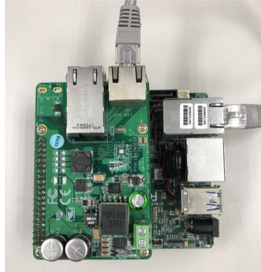
5. Connect LAN1 on PoE to LAN port on the MB with LAN cable in accessory kit.
