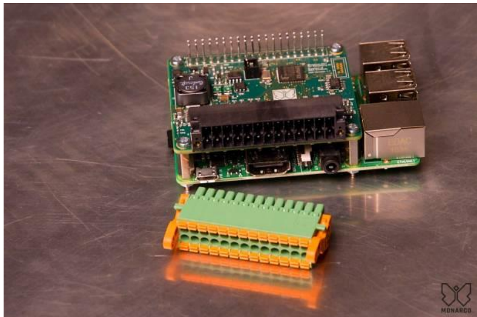
Image 1.1: Monarco HAT board mounted on Raspberry Pi, with detached terminals connector.
