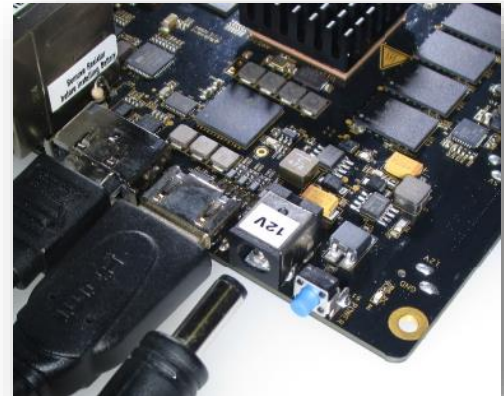
Figure 18. DC Jack Into P1
