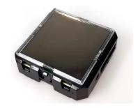
STM 550U provides an integrated NFC interface that can be used for device configuration and device commissioning and an LRN button that can be used for simple commissioning tasks.
