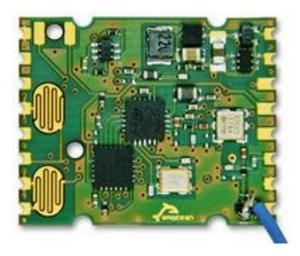
The security mode and the telegram content can be selected using six configuration interface signals.
