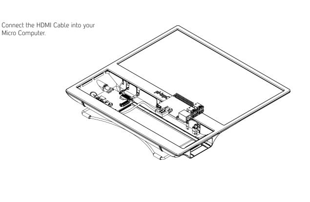
Step 6: Inserting Micro Computer
