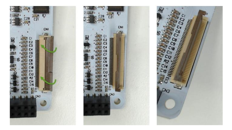
The cable terminal is the same for every screen. With the connector open, slide the cable on the beige part of the connector and gently push it so that it reaches underneath the brown clip. Make sure that the cable is inserted evenly so that when the clip is rotate back into the closed position the two dots shown in the picture are parallel with the connector.
