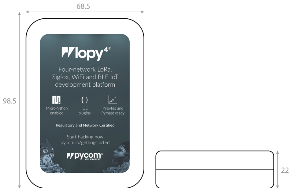
Figure 10 – Mechanical drawing of packaging – Units: mm
