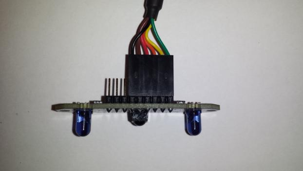
The ZX/SP sensor has labeled connections with UART and I2C separated. This makes it easy to connect ready-made connectors (like the FTDI UART connector) directly to the ZX sensor pins (as shown). Similarly, the I2C connection pins may connect to any two-wire interface using the ZX sensor as the I2C slave, and any embedded or external processor as the I2C master.
